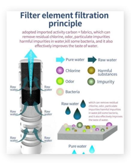
Adopts activated carbon filter and ACF+Fabrics filtration principle, which can effectively filter the water source and remove residual chlorine, odor, granular impurities and harmful substances in the water. At the same time, the filter device can also kill some bacteria, effectively improve the taste of water, and bring you a purer and healthier drinking experience.
